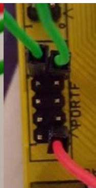
Figure 8 - Bit 6 jumper connected to bit 0 on PORT F
